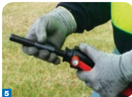
5 Larger penetration holes are achieved by fitting a larger handle into the tool.
